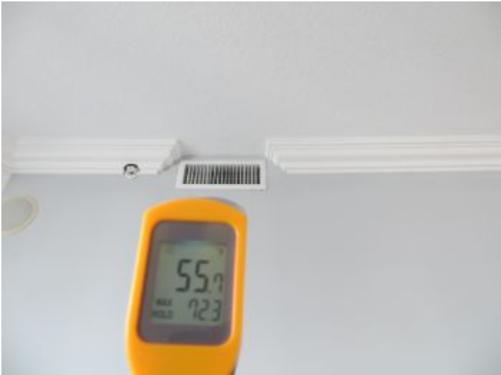
operated, Room temp ( 73°) Cold side, ( 55°)
